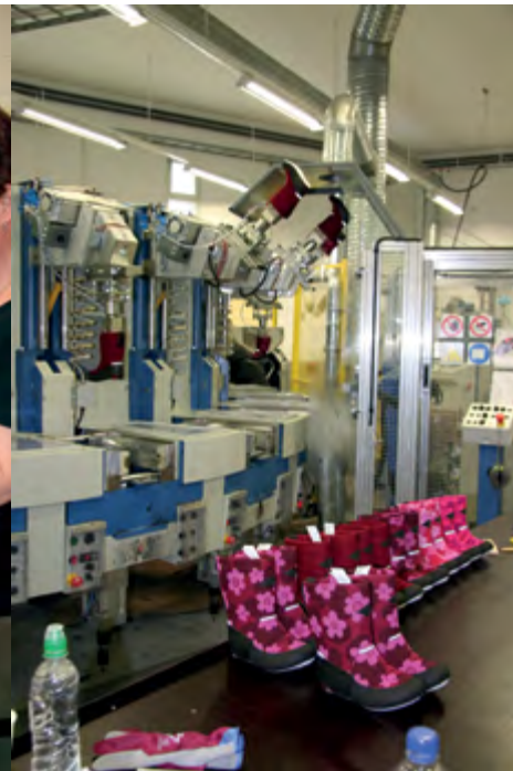
8. This machine makes the rubber soles for the shoes.
