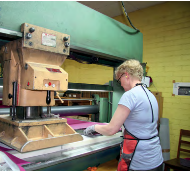
3. The punching tool cuts out the outer parts for the boot from the material according to the pattern.
