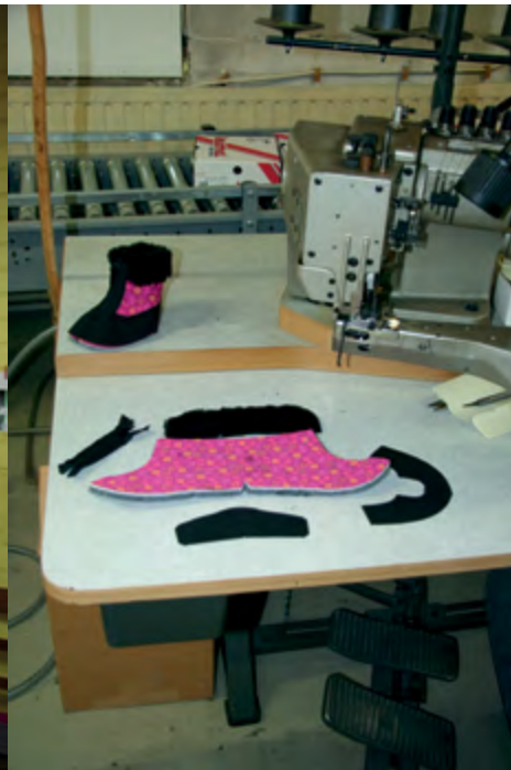
4. All of the parts that need to be sewn for the shoe are put together.
